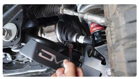
STEP 3 | Install the other (2) M8 carriage bolts and secure them in place using a 13mm wrench and the provided M8 flat washer and nylon lock nut
