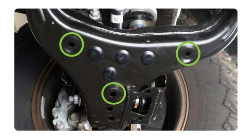
STEP 2 | Place the DV8 A-Arm skid plate against the bottom of the A-Arm while aligning the skid plate bolt holes with the holes in the A-Arm.
