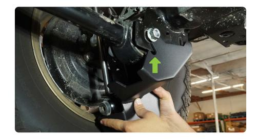
STEP 3 | Using the factory shock mount bolt secure the skid plate.
