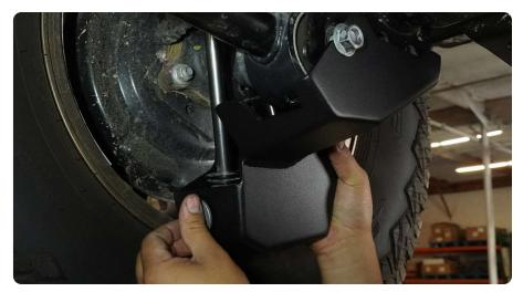
STEP 4 | Secure the shock mount bolt in the first picture using a 17mm socket. Torque to 65 ft-lbs.
