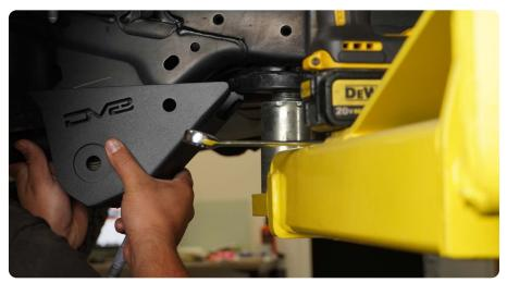
**STEP 4** | With the skid plate in position over the hole, move the trailing arm back into place.
