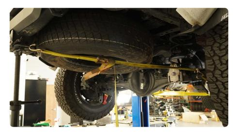
**STEP 2** Use a 19mm socket and wrench to remove the trailing arm bolt and nut.
