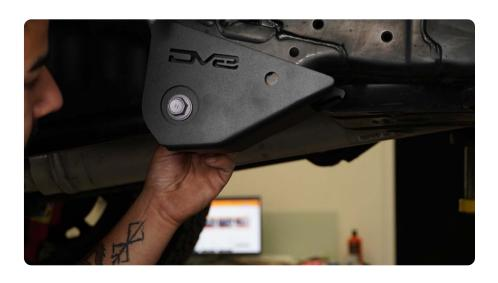
**STEP 5** Using the provided M12 bolts, install the bolt into the upper mounting hole of the skid plate though the hole on the mount.
