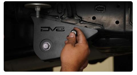
**STEP 6** Using a 18mm socket and 19mm wrench, tighten the upper bolt until secure.
