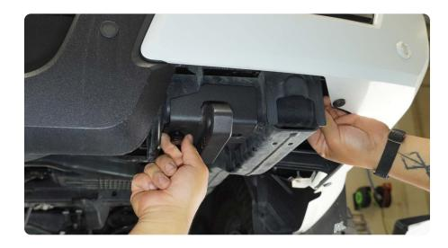
STEP 6 | TRD/SR/SR5: Secure the M12 Bolts using a 18mm socket. Do not exceed 92 ft lbs.
