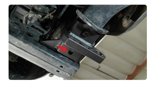
STEP 9 | SR/SR5: With both required bolts fully installed, use a marker to mark the hole that will need to be drilled into the hitch square tube.
