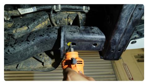
STEP 17 | TRD: Use paint to cover any bare metal to prevent rust.
