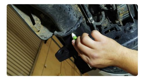
STEP 16 | TRD: Drill optional hole to 1/2" diameter, and remove marked material on non-optional hole.
