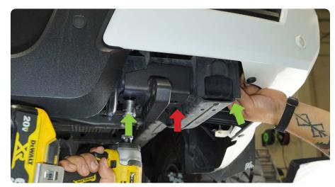
STEP 7 | TRD/SR/SR5: Secure the M14 bolt using a 21mm & 22mm socket or wrench. Do not exceed 100 ft lbs.
