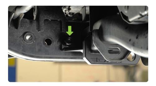
STEP 4 | TRD/SR/SR5: Install the provide nut plate into the hitches square tube. The angled handle end of the nut plate should be pointed up toward the bed.
