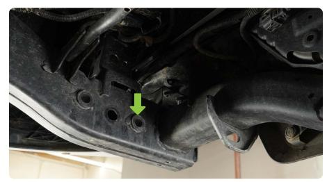
STEP 14 | TRD: Using a marker, mark the optional hole.
