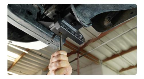
STEP 11 | SR/SR5: Use a step bit or 1/4" drill bit to drill a pilot hole.
