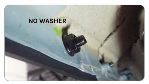
STEP 3 | Place the rear section of the covers up to the pinch welds and secure using the provided M8 hardware with a 13mm socket.
