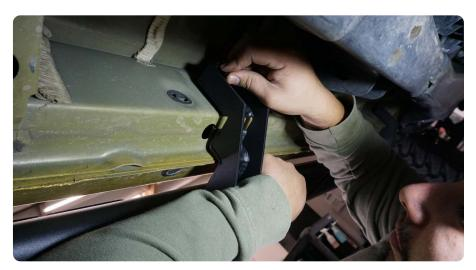
STEP 3 | These OE Plus steps have the ability to be adjusted forward and backward, adjust the steps to your liking.
