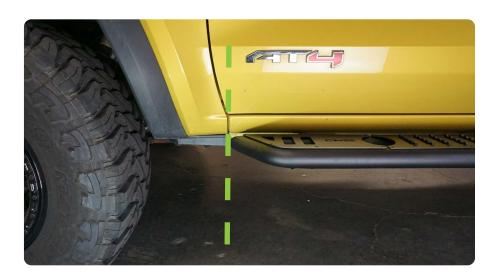
STEP 4 | Secure the steps to the vehicle using a 13mm socket.
