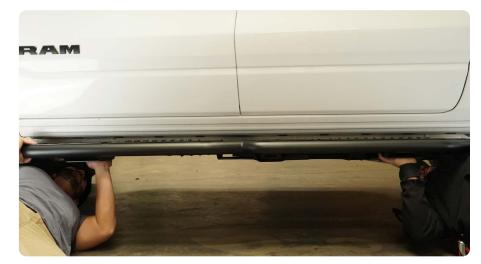
STEP 4 | Use a 13mm socket to secure all M8 hardware.
