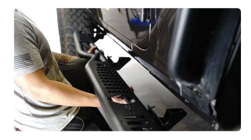
STEP 3 | Once all hardware is loosely installed, secure the hardware on the studs using a 10mm and 13mm socket.
