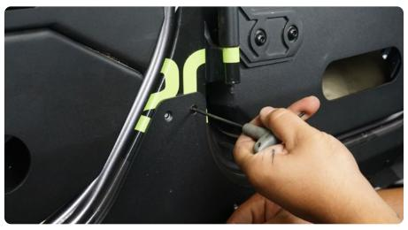
**STEP 8** | With the rock skins installed and the hardware secure, use a punch tool to mark the remaining mounting holes for drilling.
