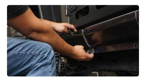
Loosely install rock skins using the provided M5 hardware. Do not secure until all hardware is partially threaded.
