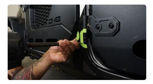
STEP 5 | Drill out the marked mounting holes using a small drill bit, working your way up to a 9/32" bit.
