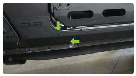
**STEP 12** | Install the provided nutserts into the remaining mounting holes using a nutsert tool (or the provided nutsert tool, if you do not have one).
