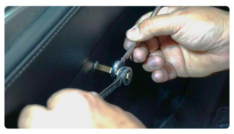
STEP 18 Use a 12mm wrench to hold the spacer while tightening with a 10mm socket. Tighten slowly until the nutsert is set properly. Do not over tighten.
