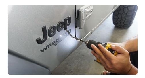
STEP 10 | Install the provided nutserts into the remaining mounting holes using a nutsert tool (or the provided nutsert tool, if you do not have one).
