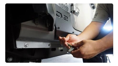
STEP 8 | With the rock skins installed and the hardware secure, use a punch tool to mark the remaining mounting holes for drilling.
