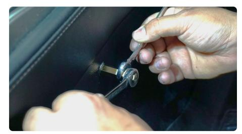
STEP 15 | Use a 12mm wrench to hold the spacer while tightening with a 10mm socket. Tighten slowly until the nutsert is set properly. Do not over tighten.
