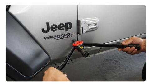
Loosely install rock skins using the provided M5 hardware. Do not secure until all hardware is partially threaded.
