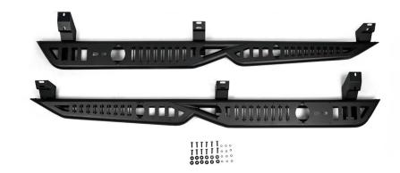
STEP 1 | with assistance, lift the DV8 OE plus step up to the vehicle and align the mounting brackets with the (8) factory threaded holes in the rocker panel.
