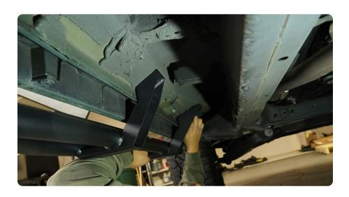
$\begin{array}{c|c} \text{STEP 2} & \text{Center the steps side to side} \\ \text{with the vehicle.} \end{array}$
