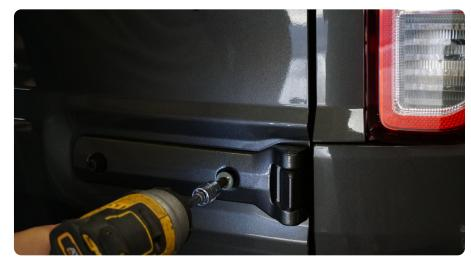
STEP 4 Use a 13mm socket to remove the eight bolts securing the factory spare tire carrier to the vehicle.
