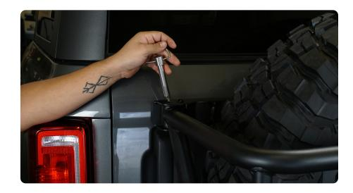
STEP 13 | Install the provided M8x75 hardware next to the pin using a 5mm allen bit and secure. This will help to prevent any rattling from up and down movement of the carrier in the latch area.
