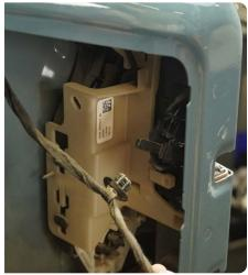
STEP 22 | Use a trim clip tool to remove the harness connector plugs from the tailgate.
