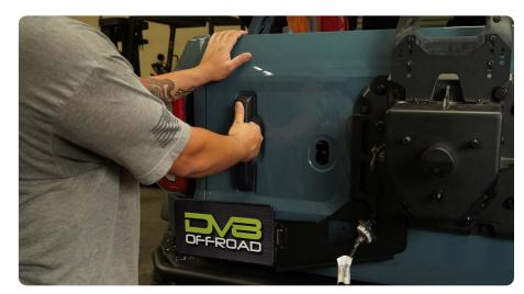
$\begin{array}{c|c} \text{STEP 37} & \text{Ensure the tailgate is flush} \\ \text{with the vehicle body.} \end{array}$
