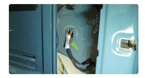
STEP 3 | Use a 13mm socket to remove the factory spare tire mount.
