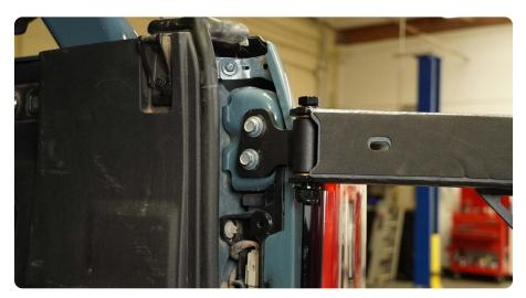
STEP 34 | With assistance, have one person hold up the tailgate up to the DV8 tire carrier while the second person installs the (4) provided M8x40 tailgate hex bolts using a 13mm socket.
