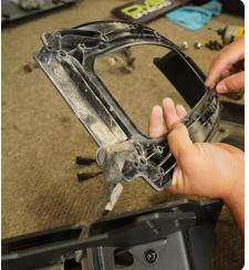
STEP 15 | Reassemble the third brake light housing using a T25 torx tool.
