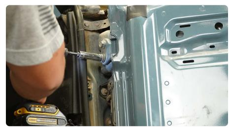
STEP 29 | Use a T47 torx tool to remove the factory hinges from the tailgate.
