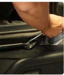
STEP 20 | Use a trim clip tool along the bottom to remove the trim cover panels on the tailgate. Be careful not to damage any retaining clips.
