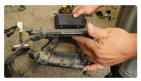
STEP 13 | Remove the third brake light harness from the brake lights housing.
