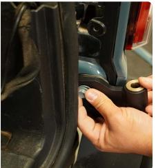
STEP 32 | Install the top hinge without any shims as shown.
