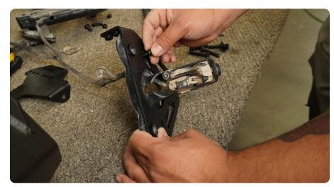
STEP 9 | Carefully install the rear camera housing into the DV8 spare tire mount.
