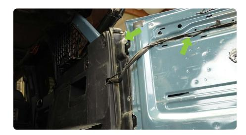
STEP 45 | Reconnect the latch sensor harness, rear camera harness, and third brake light harness.
