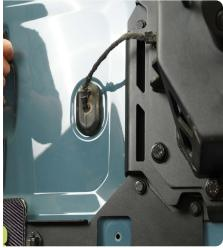
STEP 44 | Reinstall the interior factory wiring harness and hinge bolt cover in the reverse order they were removed.
