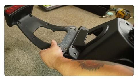
STEP 5 Use a T30 torx tool to remove the (2) bolts securing the factory wheel stud plate.
