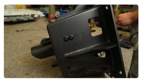
STEP 11 | Mount the third brake light mounting bracket to the DV8 spare tire mount using (2) M6x20 Allen head bolts, (2) M6 serrated nuts, a #4 Allen tool and 10mm wrench.
