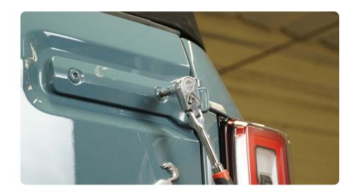
STEP 26 | Use a Phillips head screwdriver to remove the (4) push pins retaining the main hinge cover.
