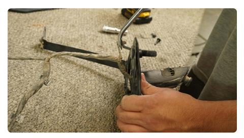
STEP 7 Use a T20 torx tool to remove the rear camera from its housing.
