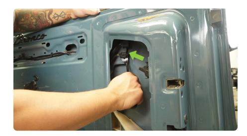
STEP 23 | Pull the wiring harness back through the tailgate while using the trim clip tool to remove any harness clips retaining the wiring harness to the tailgate.
