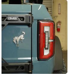
STEP 39 | With the tailgate to body gaps even, secure the (12) tire carrier to tailgate bolts hand tight using a 13mm socket.
