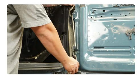
STEP 28 | Use a 13mm socket and a ratchet wrench to break loose the (4) hinge to vehicle body bolts.
