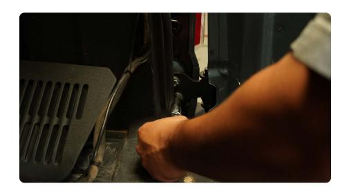
STEP 38 | Check the tailgates side to side gap. If they look as shown on either side adjust the tailgate with a firm grip in the direction needed to evenly space out tailgate to vehicle body gaps. Move the side to side with the door latched.
