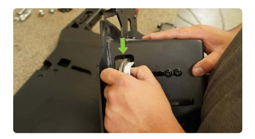
STEP 17 | Mount the spare tire mount on to the DV8 tailgate bracket using (8) of the provided M14x35mm hex bolts and a 21mm socket.
