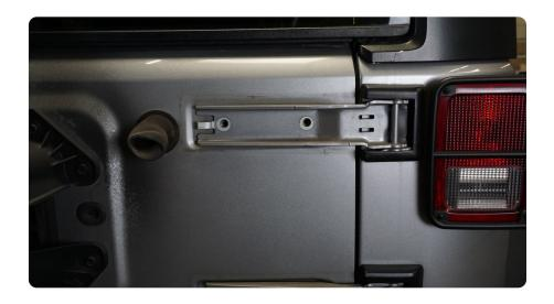
STEP 4 Using the M8x30 hex head bolts, install the top mounting bracket to the top hinge until secure using a 13mm socket.
