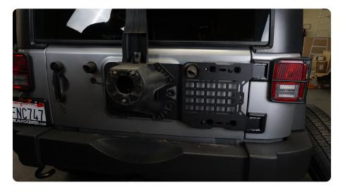
STEP 11 | Tighten the hinge mounting hardware using a #5 allen head.
