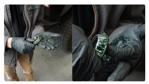
**STEP 15** Install one of the provided bearing/race sets into the bottom of the tire carrier.
