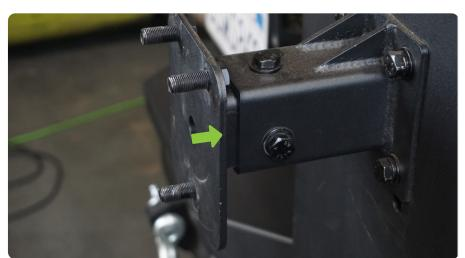
**STEP 32** | Secure the tire carrier portion of the asembly using a 16mm socket.
