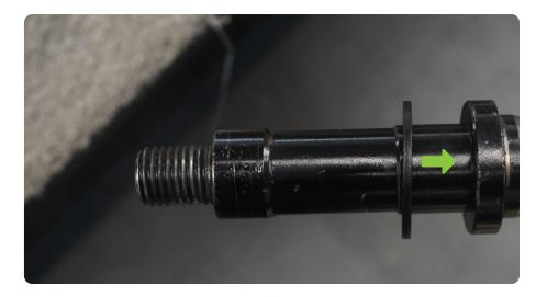
STEP 18 | Install one of the provided bearing/race sets into the top of the tire carrier.
