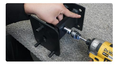
STEP 25 | Slide the large square nutplate into the swing arm of the tire carrier, and secure the main tire carrier assembly to the swing arm using the provided M10x35 hardware with a 16mm socket.
