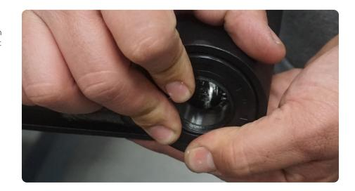
STEP 17 | Install the larger provided black washer onto the top of the spindle.
