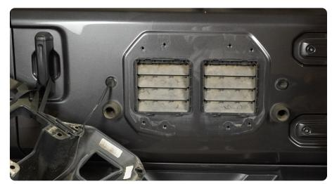
STEP 8 | Unpeel the foam provided and place it onto the backside of the carrier molle.
