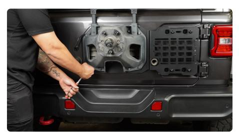
STEP 11 | Tighten the hinge mounting hardware using a #6 allen head.
