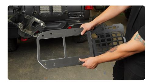
STEP 9 | Hold the panel up to the hinges installed earlier and align the nutserts on the hinges to the slots on the panel.
