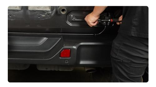
STEP 4 Using the M10x40 hex head bolts, install the bottom mounting bracket to the bottom hinge until secure using a 16mm socket.
