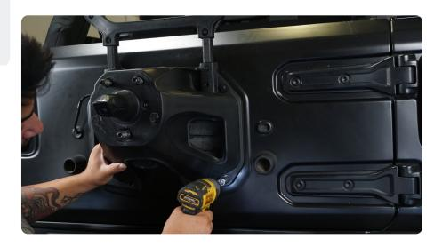
**STEP 2** Use a T25 torx bit to remove the hardware securing the third brake light to the tire carrier.
