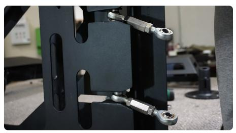
STEP 11 | Loosely install the stopper bracket using the provided M10x25 hardware.
