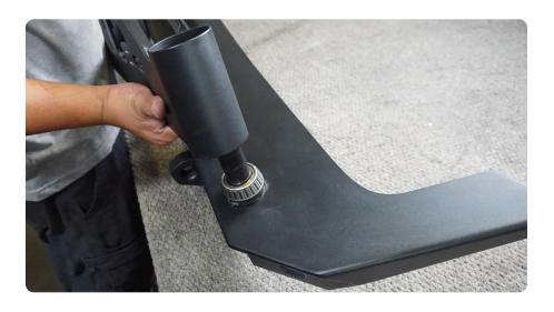
**STEP 19** Install the upper race and remaining bearing as shown with the race being placed first, and the bearing on top, facing down.
