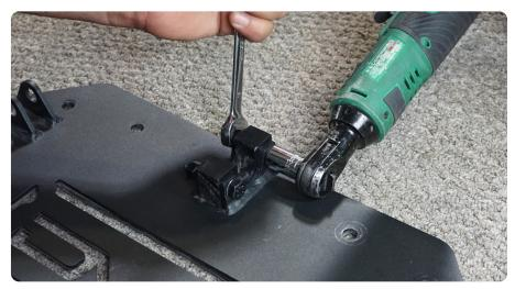
**STEP 13** | Install the backing plate to the tailgate of the vehicle using the factory hardware and a 13mm socket.
