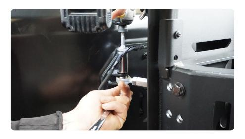
**STEP 33** Adjust the heim joints by turning the center connector nut.
