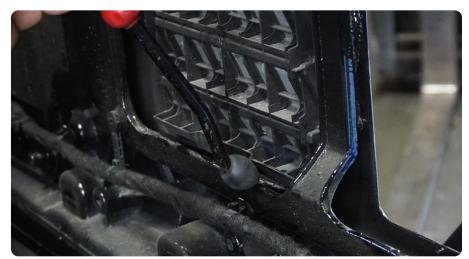
**STEP 8** Using a Dremel or cutting tool of choice, remove the three sided border from the fin vents.
