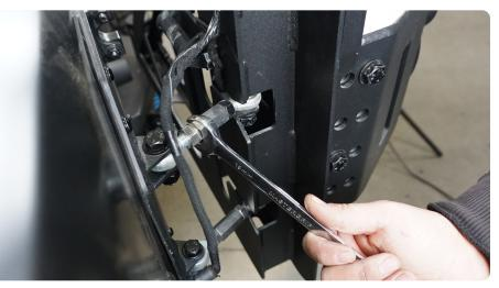
**STEP 34** | Check and adjust the tire catch up/down so that the stopper lands in it when the tailgate is closed.
