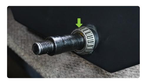
**STEP 16** | Place the tire carrier on to a work bench upside down. Place the lower bearings race into the tire carrier as shown.
