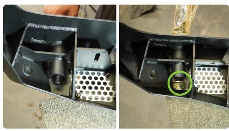
**STEP 15** | Install the provided spacer plate, followed by the bearing as shown.
