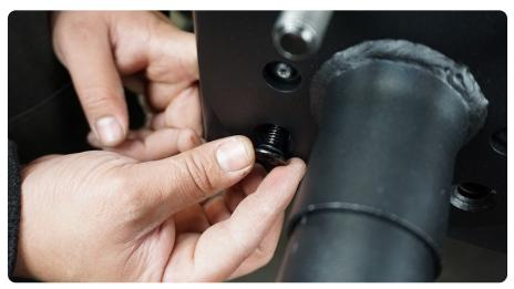
STEP 31 | Adjust the camera tube and secure using the provided M6 hardware with a #4 Allen bit.
