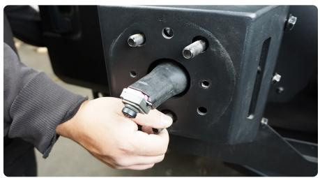
STEP 28 | Secure the factory rear camera/ tire mount to the DV8 Tire Carrier using the (2) factory torx head screws previously removed.
