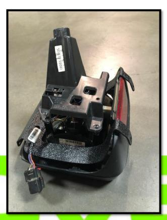
4. Slide the light and backing bracket into the tail light guard as shown below. Install screws loosely.
