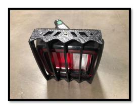
5. Once both lights are built, connect the wiring and place them back into the holes for reinstallation. With the tail light guard housing loose, you can align them perfectly before placing the factory light bolt into light.
