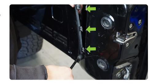
STEP 3 | Disconnect the third brake light wiring harness. Small gray plug shown in image.
