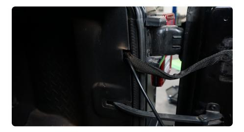
Push factory License plate light wiring harness back through the body hole and up into the trunk area of vehicle.
