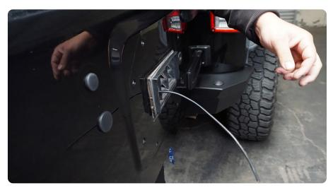
STEP 10 | Unravel the third brake light factory wiring harness previously disconnected in step 3.
