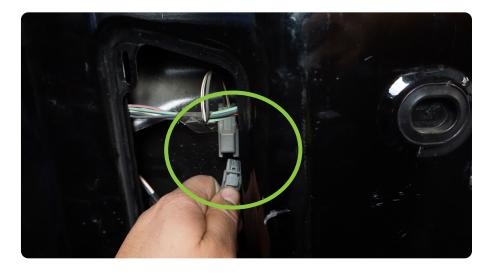
STEP 4 | With the light unplugged, push the rubber grommet holding the wire towards the outside (back) of the vehicle.
