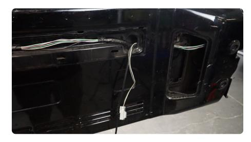
STEP 12 | Cut the factory third brake light wiring harness plug off.
