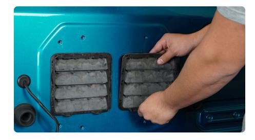
$\begin{array}{c|c} \text{STEP 17} & \text{Place the provide foam} \\ \text{piece on to the body mounting plate.} \end{array}$
