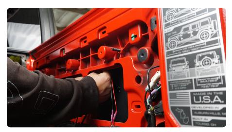
STEP 29 | Use the provided rubber plugs to seal the factory tail gate holes.
