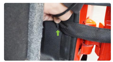
STEP 32 | Route the DV8 License plate light harness under the carpet and over to the drivers side.
