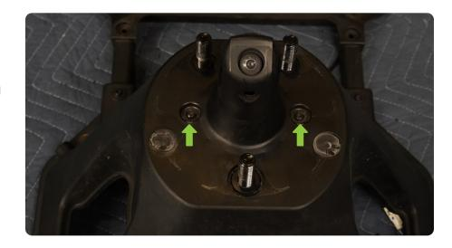
STEP 10 | To remove the stud plate, tap on the studs evenly with a hammer or mallet to push them through the carrier. The stud plate should fall away from the camera mount and carrier.
