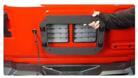
STEP 25 | Push the factory wiring harness back through the hole in the tailgate.
