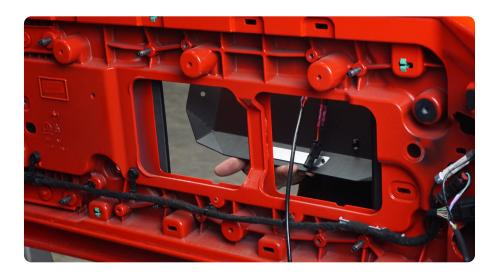
STEP 27 | Using the provided M6 hardware and a #4 Allen bit, mount the spare tire face plate to the body mounting plate.
