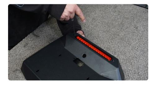
STEP 19 | Mount the provided license plate light using the provided M4 Philips head hardware and lock nuts.
