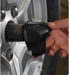
STEP 2 | Remove your spare wheel/ tire. Factory lug nuts are a 22mm socket.
