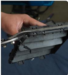
STEP 16 | Replace the vents into the door by clipping them into place from the outside pushing towards the inside.
