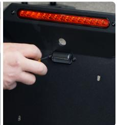
STEP 20 | Use the provided M6 hardware and an #4 Allen bit to mount the license plate.
