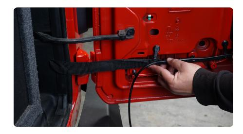
STEP 31 | Push the DV8 license plate wiring harness down and behind the interior trim so that it can be pulled from under the carpet.
