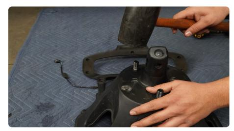
STEP 11 | Once free, using a socket or in our case a 3/8" socket extension, we tapped lightly on the exposed camera mounts in each stud hole. We also reinserted each T25 screw just to the left and right of the camera tower and tapped on these. The camera mount is not glued but pressed in slightly so some light force may be needed to release it.
