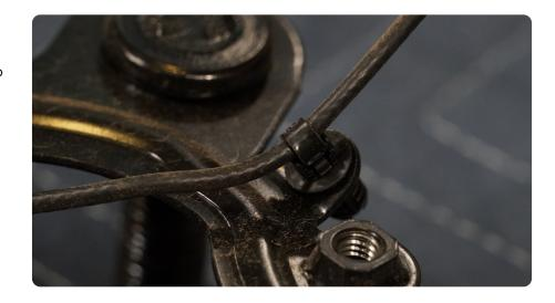
STEP 13 | Pull the camera mount from the carrier and using a T8 Torx bit, remove the camera from the mount and unplug from the harness and set everything off to the side.
