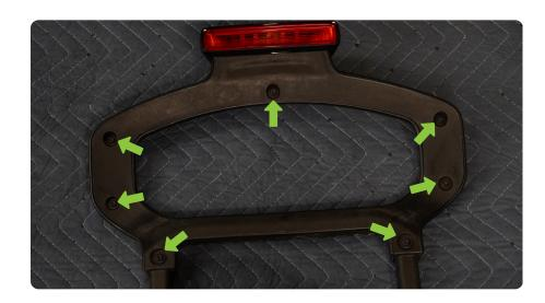
STEP 8 | Split the front and back of the third brake light housing to gain access to the light mount and the plug. Using the same T25, remove the two bolts holding the light and then unplug the light from the harness. Set all components off to the side.
