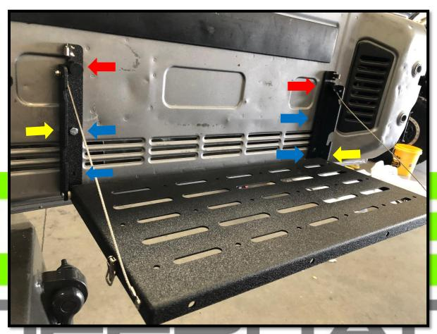
7. Drill hole to 5/16 and insert nutserts. (NOTE: Nutserts have to be installed into the metal properly. If you are not experienced with nutserts please research online prior to installation).
