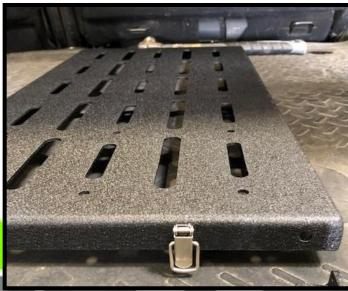
2. Install the table wires into shown holes on each side using provided hardware.
