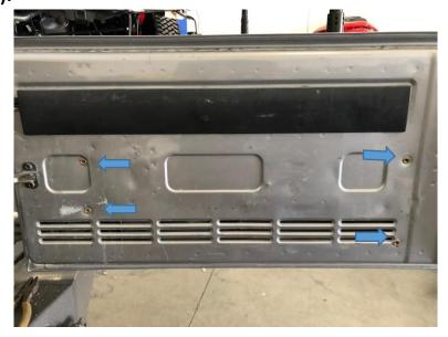
8. Install table using provided hardware and metal stops on top nutserts as shown. Cover with rubber pads.
