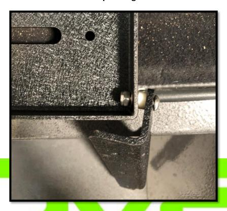
5. Hold table against rear hatch. Choose desired location of table and hold in place to mark holes. We used a large clamp and a second sent of hand to make this much easier.
