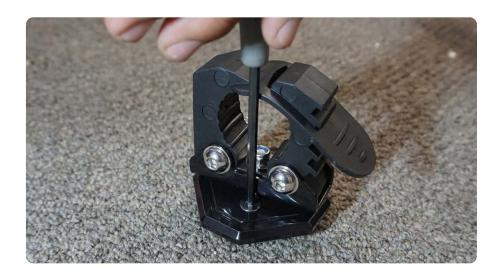
STEP  $2 \mid$  with the screws removed the back should come off.
