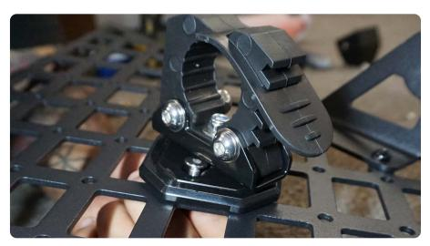
STEP 4 Using the #4 allen head, secure hardware.
