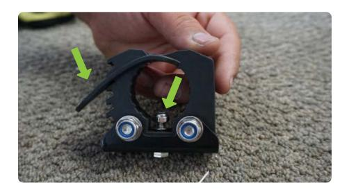
STEP 2 Using a 10mm socket on the nut side, and a 10mm wrench/socket on the bolt head side, remove the bolt from the mount.
