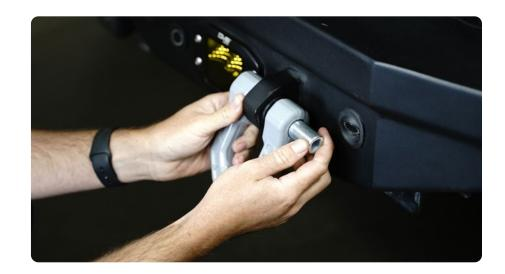
STEP 4 Using a 3/8" ratchet/chuck, being to tighten the pin into the shackle until secure. The pin should be tight enough that the pin cannot be loosened by hand.
