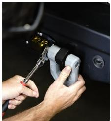
STEP 5 Double check both pins are secure, and you are ready to put your new Elite Series D-Ring to the test!
