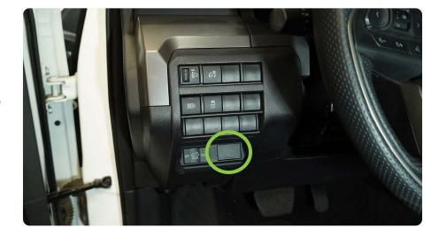
STEP 2 | Remove the blank accessory switch cover and use an 3/4" drill bit or step bit to drill out a 3/4" hole.
