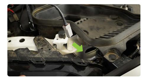
STEP 9 | Route the positive/negative ring terminals, relay and fuse-able link towards the vehicles battery.
