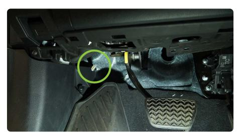
STEP 7 | Connect the Switch and main harness back together.
