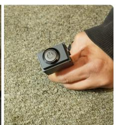
STEP 5 | Reinstall the accessory cover and switch back into the slot it was removed from.
