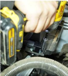
STEP 11 | Reinstall any trim panels and double check for any loose wiring.
