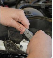
STEP 5 | Double check that all wiring is clear of any rotating or hot engine components.
